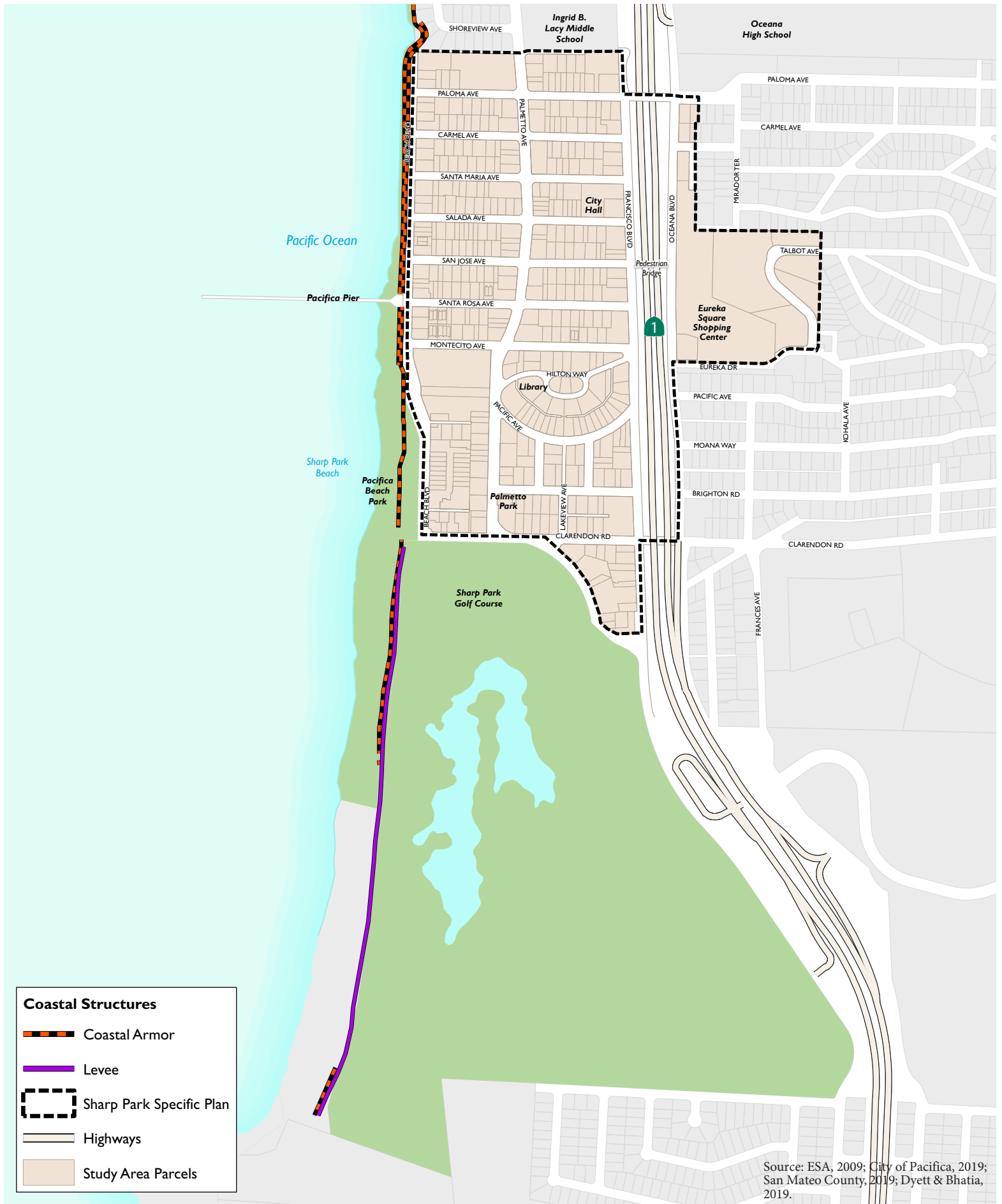
Figure 6-6: Sharp Park Coastal Protection Structures
