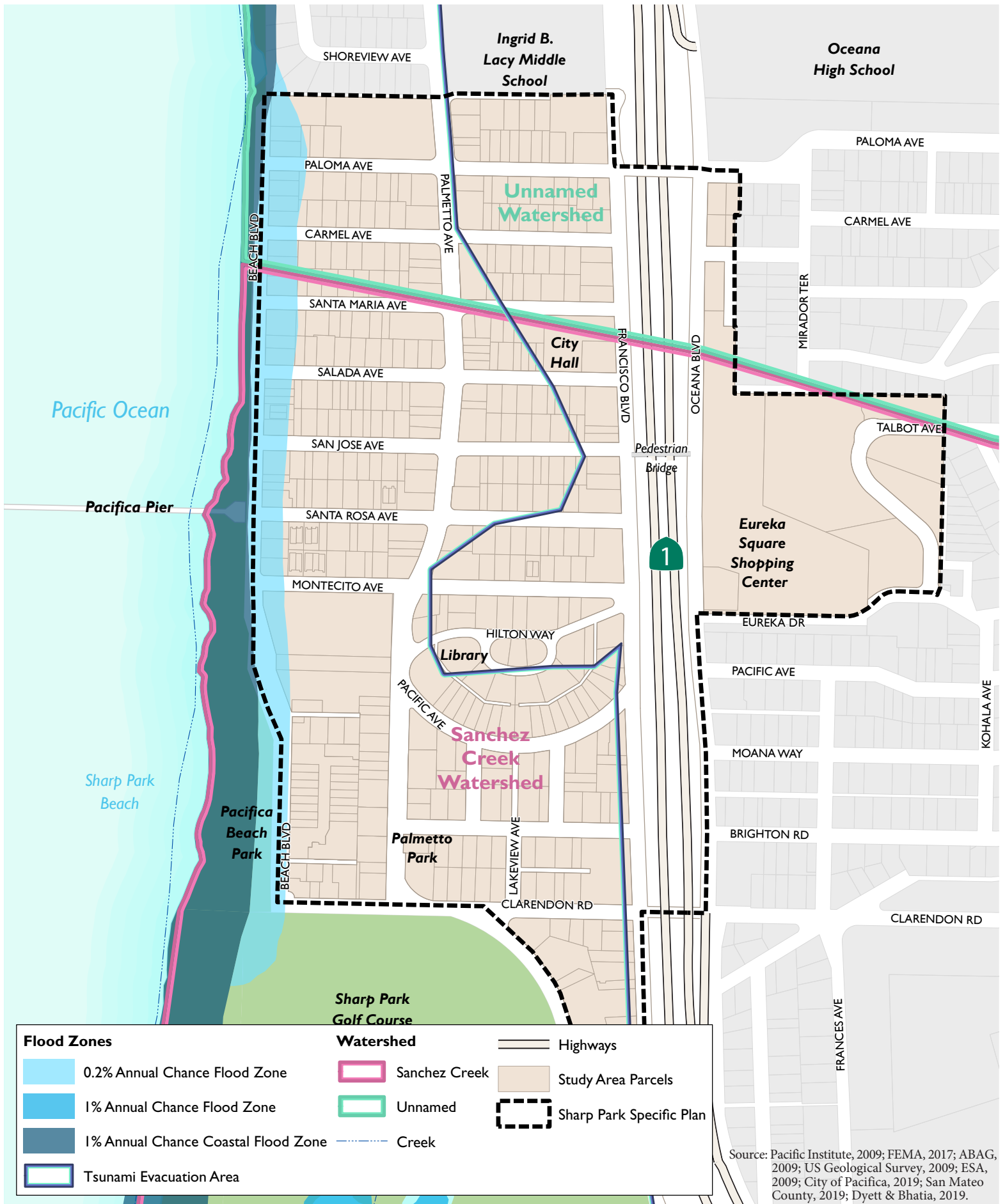
Figure 6-7: Sharp Park Hydrology and Floodzones
